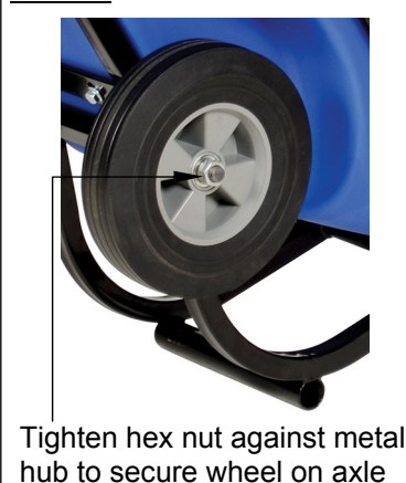
FIG. 1B: Attach wheels to axle
