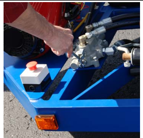
Fig. 7: Compactor orientation control
