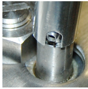
FIG. 4: Spline & Roll Pin Connection
