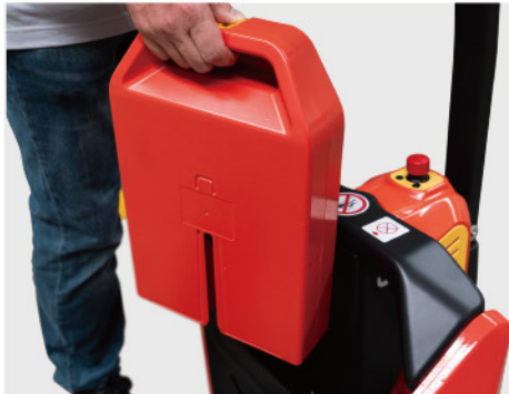
Light weight high quality Lithium battery for easy replacement .
