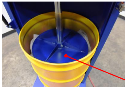
Platen compacts drum contents
