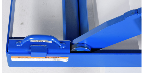
Install maintenance stops in corners of base frame
