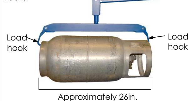
FIG. 5: Grasp cylinder with load hooks
